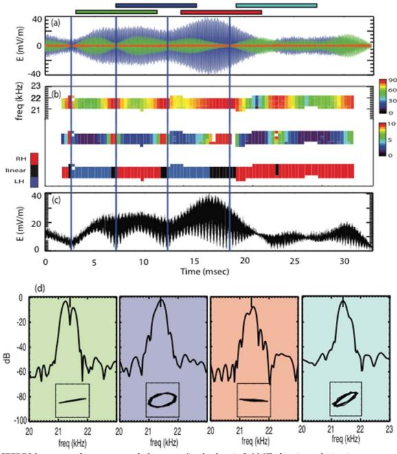
STEREO burst waveform capture of a large amplitude electric field (*E*) showing polarization reversals. This particular waveform is a whistler mode wave associated with the ground transmitter call sign NPM, detected during a STEREO Earth-flyby on November 6<sup>th</sup>, 2006.
